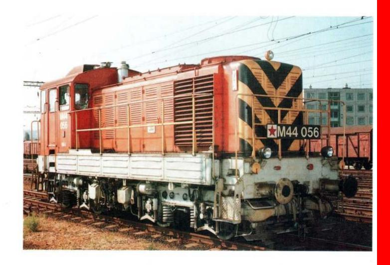
Class M44 (at the beginning marked as M424) is a Diesel locomotive with electric transmission system and the first unit of her was commissioned in 1954. This locomotive was in that time the most powerful Diesel locomotive of the MÁV, designed and manufactured by MÁVAG later by Ganz-MÁVAG. She was intended for the light goods trains and medium shunting service. The Diesel engine built into this locomotive drives a D.C. main generator
