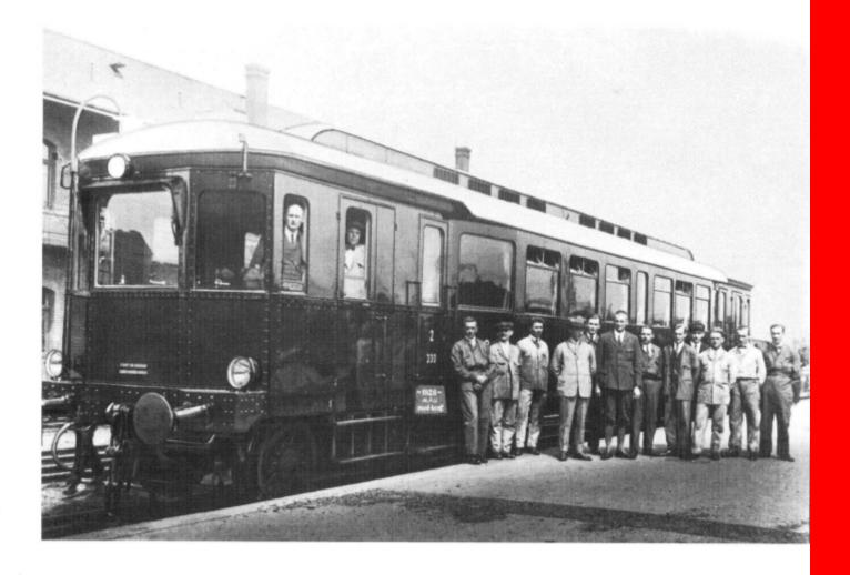
This experimental railcar (later marked with nameplate No. 304) was built in 1926 by the German Eisenbahn Verkehrsmittel AG (EVA) company (i.e.: Railway Vehicle Company). The Maybach-type Diesel engine built in this railcar was the most up-to-date model in the middle 1920's. The power pack was accomodated in one of the bogies. The mechanical transmission (change gear) drove a dummy shaft through a bevel-geared reversing gear. The four
