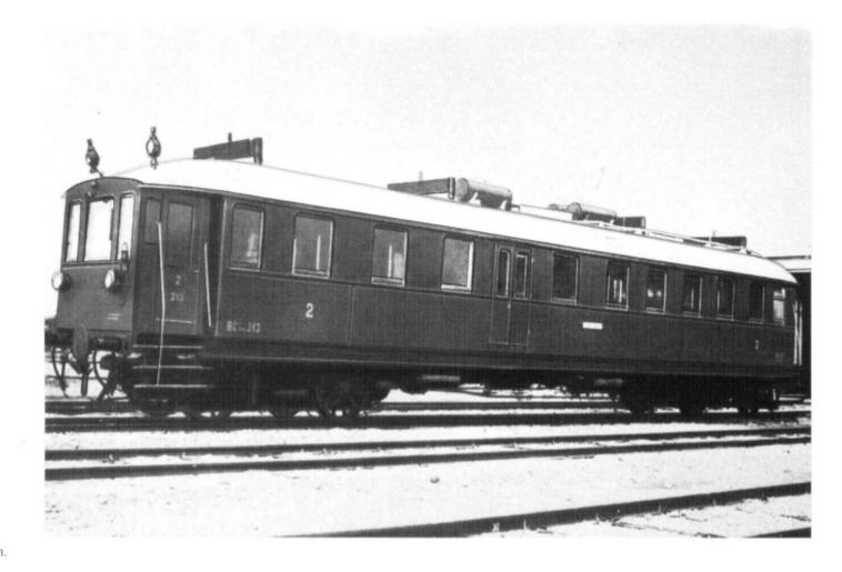
In 1926 MÁV had three 4-axled railcars built. These railcars were built by using up and strenghtening the underframes of former 4-axled steam engine powered railcars by MÁVAG and MÁV Istvántelki Főműhely (i.e. overhaul shop of MÁV at Istvántelek) and got nameplate No-s 311, 312 and 313. The railcars were equipped with two complete power packs composed of engine, mechanical speed change gear and axle drive, each being identical with that
