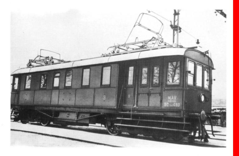
On the electrified local railway of Vác-Budapest-Gödöllő, maintained by MÁV, the passenger traffic was performed with electric ralicars. The vehicle part of the Class ACa railcar was built by the Magyar Waggon- és Gépgyár Rt. (i.e. Hungarian Wagon- and Machine Works Company) of Győr while the electric part was manufactured by the Magyar Siemens-Schuckert Művek Kft. (i.e. Hungarian Siemens-Schuckert Works Ltd) of Budapest and Pozsony
