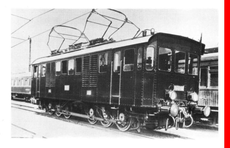
MÁV placed the order in 1931 with Ganz works to deliver the Class V60 locomotives to maintain the heavy goods trains on the mainline Budapest-Hegyeshalom. The electric equipment of these locomotives was identical with that of the Class V40 locomotives. The difference between of the two Class of locomotives was in the vehicle part built by MÁVAG, namely in the main frame, in the running gear and in the transmision gear. The running gear construction
